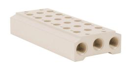
NITRA pneumatic valve manifold, aluminum, off-white, (6) stations, (2) 1/4in female NPT inlet(s), (4) 1/4in female NPT exhaust(s). For use with AVS-51 series directional control valves.
