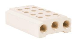
NITRA pneumatic valve manifold, aluminum, off-white, (4) stations, (2) 1/4in female NPT inlet(s), (4) 1/4in female NPT exhaust(s). For use with AVS-51 series directional control valves.
