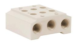
NITRA pneumatic valve manifold, aluminum, off-white, (2) stations, (2) 1/4in female NPT inlet(s), (4) 1/4in female NPT exhaust(s). For use with AVS-51 series directional control valves.
