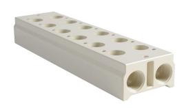
NITRA pneumatic valve manifold, aluminum, (6) stations, (2) 3/8in female NPT inlet(s), (2) 3/8in female NPT exhaust(s). For use with AVS-33 series directional control valves.
