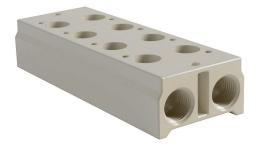
NITRA pneumatic valve manifold, aluminum, off-white, (4) stations, (2) 3/8in female NPT inlet(s), (2) 3/8in female NPT exhaust(s). For use with AVS-33 series directional control valves.
