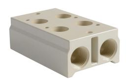
NITRA pneumatic valve manifold, aluminum, off-white, (2) stations, (2) 3/8in female NPT inlet(s), (2) 3/8in female NPT exhaust(s). For use with AVS-33 series directional control valves.
