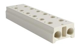
NITRA pneumatic valve manifold, aluminum, off-white, (6) stations, (2) 1/4in female NPT inlet(s), (2) 1/4in female NPT exhaust(s). For use with AVS-32 series directional control valves.
