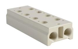
NITRA pneumatic valve manifold, aluminum, (4) stations, (2) 1/4in female NPT inlet(s), (2) 1/4in female NPT exhaust(s). For use with AVS-32 series directional control valves.
