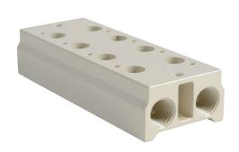
NITRA pneumatic valve manifold, aluminum, off-white, (4) stations, (2) 1/4in female NPT inlet(s), (2) 1/4in female NPT exhaust(s). For use with AVS-32 series directional control valves.
