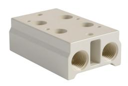
NITRA pneumatic valve manifold, aluminum, off-white, (2) stations, (2) 1/4in female NPT inlet(s), (2) 1/4in female NPT exhaust(s). For use with AVS-32 series directional control valves.
