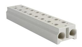
NITRA pneumatic valve manifold, aluminum, off-white, (8) stations, (2) 1/4in female NPT inlet(s), (2) 1/4in female NPT exhaust(s). For use with AVS-31 series directional control valves.
