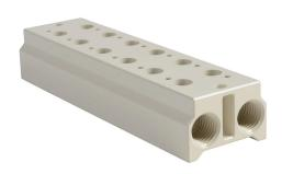
NITRA pneumatic valve manifold, aluminum, off-white, (6) stations, (2) 1/4in female NPT inlet(s), (2) 1/4in female NPT exhaust(s). For use with AVS-31 series directional control valves.
