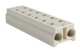
NITRA pneumatic valve manifold, aluminum, (6) stations, (2) 1/4in female NPT inlet(s), (2) 1/4in female NPT exhaust(s). For use with AVS-31 series directional control valves.
