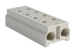
NITRA pneumatic valve manifold, aluminum, off-white, (4) stations, (2) 1/4in female NPT inlet(s), (2) 1/4in female NPT exhaust(s). For use with AVS-31 series directional control valves.
