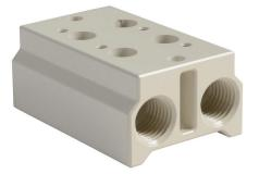
NITRA pneumatic valve manifold, aluminum, off-white, (2) stations, (2) 1/4in female NPT inlet(s), (2) 1/4in female NPT exhaust(s). For use with AVS-31 series directional control valves.
