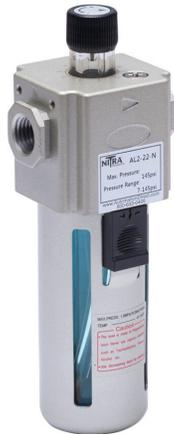
NITRA pneumatic lubricator, 1/4in female NPT inlet(s), 1/4in female NPT outlet(s), nylon bowl, metal bowl guard. For use with Ax-22 series air prep components.
