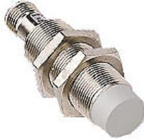
Micro Detectors inductive proximity sensor, tubular, 18mm diameter x 64mm body, nickel-plated brass housing, PNP, N.O. output, 12mm sensing distance, non-flush, 300 Hz switching frequency, IP67, 4-pin M12 quick-disconnect.
