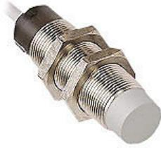
Micro Detectors inductive proximity sensor, tubular, 18mm diameter x 50mm body, nickel-plated brass housing, PNP, N.O. output, 12mm sensing distance, non-flush, 300 Hz switching frequency, IP67, pigtail.
