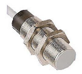
Micro Detectors inductive proximity sensor, tubular, 18mm diameter x 50mm body, nickel-plated brass housing, PNP, N.O. output, 5mm sensing distance, flush, 600 Hz switching frequency, IP67, pigtail.
