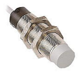
Micro Detectors inductive proximity sensor, tubular, 18mm diameter x 50mm body, nickel-plated brass housing, NPN, N.O. output, 12mm sensing distance, non-flush, 300 Hz switching frequency, IP67, pigtail.
