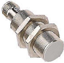
Micro Detectors inductive proximity sensor, tubular, 18mm diameter x 64mm body, nickel-plated brass housing, NPN, N.O. output, 5mm sensing distance, flush, 600 Hz switching frequency, IP67, 4-pin M12 quick-disconnect.
