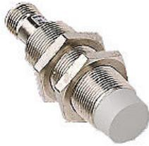
Micro Detectors inductive proximity sensor, tubular, 18mm diameter x 64mm body, nickel-plated brass housing, NPN/PNP, N.O. output, 8mm sensing distance, non-flush, 300 Hz switching frequency, IP67, 4-pin M12 quick-disconnect.
