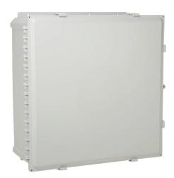
AttaBox Heartland series enclosure, with shelf, NEMA 1/3R/4/4X/12, 24 x 24 x 10in (HxWxD), wall mount, polycarbonate, Pantone 7541 C light gray, single-door, polycarbonate quick-release latch.
