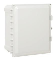
AttaBox Heartland series enclosure, with shelf, NEMA 1/3R/4/4X/12,  $12 \times 10 \times 6$ in (HxWxD), wall mount, polycarbonate, Pantone 7541 C light gray, single-door, polycarbonate quick-release latch.
