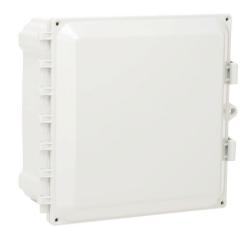
AttaBox Heartland series enclosure, with shelf, NEMA 1/3R/4/4X/12,  $10 \times 10 \times 6$ in (HxWxD), wall mount, polycarbonate, Pantone 7541 C light gray, single-door, polycarbonate quick-release latch.
