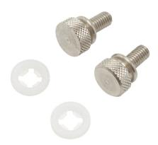
AttaBox thumb screw, replacement, #10-32 UNF x 0.375in, stainless steel. Package of 2. For use with Heartland series enclosures. Nylon washer included.
