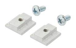
AttaBox slot nut kit, #10-32 UNF x 0.375in, Phillips pan head, zinc plated steel. Package of 2. For use with Heartland series enclosures. Includes screw and galvanized steel slot nut.
