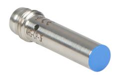
Micro Detectors inductive proximity sensor, tubular, 6.5mm diameter x 29.4mm body, stainless steel housing, PNP, N.C. output, 2mm sensing distance, flush, 7 kHz switching frequency, IP67, 3-pin M8 quick-disconnect.
