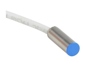
Micro Detectors inductive proximity sensor, tubular, 6.5mm diameter x 20.3mm body, stainless steel housing, PNP, N.C. output, 2mm sensing distance, flush, 7 kHz switching frequency, IP67, pigtail.
