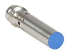
Micro Detectors inductive proximity sensor, tubular, 6.5mm diameter x 29.4mm body, stainless steel housing, PNP, N.C. output, 1.5mm sensing distance, flush, 7 kHz switching frequency, IP67, 3-pin M8 quick-disconnect.
