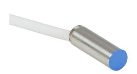
Micro Detectors inductive proximity sensor, tubular, 6.5mm diameter x 20.3mm body, stainless steel housing, PNP, N.C. output, 1.5mm sensing distance, flush, 7 kHz switching frequency, IP67, pigtail.
