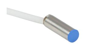
Micro Detectors inductive proximity sensor, tubular, 6.5mm diameter x 20.3mm body, stainless steel housing, PNP, N.C. output, 1.5mm sensing distance, flush, 7 kHz switching frequency, IP67, pigtail.
