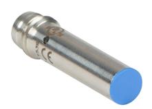
Micro Detectors inductive proximity sensor, tubular, 6.5mm diameter x 29.4mm body, stainless steel housing, PNP, N.O. output, 2mm sensing distance, flush, 7 kHz switching frequency, IP67, 3-pin M8 quick-disconnect.
