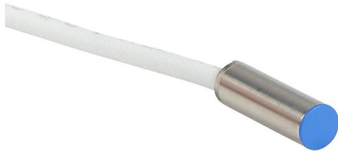
Micro Detectors inductive proximity sensor, tubular, 6.5mm diameter x 20.3mm body, stainless steel housing, PNP, N.O. output, 2mm sensing distance, flush, 7 kHz switching frequency, IP67, pigtail.
