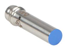
Micro Detectors inductive proximity sensor, tubular, 6.5mm diameter x 29.4mm body, stainless steel housing, PNP, N.O. output, 1.5mm sensing distance, flush, 7 kHz switching frequency, IP67, 3-pin M8 quick-disconnect.
