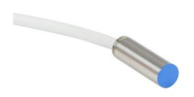
Micro Detectors inductive proximity sensor, tubular, 6.5mm diameter x 20.3mm body, stainless steel housing, PNP, N.O. output, 1.5mm sensing distance, flush, 7 kHz switching frequency, IP67, pigtail.
