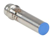
Micro Detectors inductive proximity sensor, tubular, 6.5mm diameter x 29.4mm body, stainless steel housing, NPN, N.O. output, 2mm sensing distance, flush, 7 kHz switching frequency, IP67, 3-pin M8 quick-disconnect.
