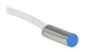
Micro Detectors inductive proximity sensor, tubular, 6.5mm diameter x 20.3mm body, stainless steel housing, NPN, N.O. output, 2mm sensing distance, flush, 7 kHz switching frequency, IP67, pigtail.
