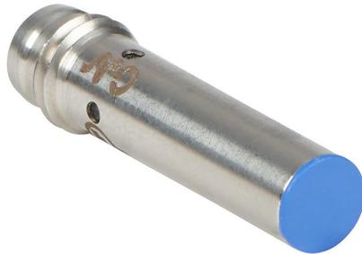
Micro Detectors inductive proximity sensor, tubular, 6.5mm diameter x 29.4mm body, stainless steel housing, NPN, N.O. output, 1.5mm sensing distance, flush, 7 kHz switching frequency, IP67, 3-pin M8 quick-disconnect.
