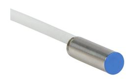
Micro Detectors inductive proximity sensor, tubular, 6.5mm diameter x 20.3mm body, stainless steel housing, NPN, N.O. output, 1.5mm sensing distance, flush, 7 kHz switching frequency, IP67, pigtail.
