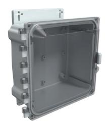
AttaBox Heartland series enclosure, NEMA 1/3R/4/4X/12, 8 x 8 x 4in (HxWxD), wall mount, polycarbonate, Pantone 7541 C light gray, smoked polycarbonate single-door, polycarbonate quick-release latch.
