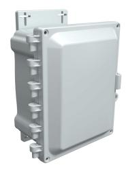
AttaBox Heartland series enclosure, NEMA 1/3R/4/4X/12, 8 x 6 x 4in (HxWxD), wall mount, polycarbonate, Pantone 7541 C light gray, single-door, polycarbonate quick-release latch.
