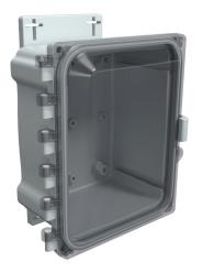
AttaBox Heartland series enclosure, NEMA 1/3R/4/4X/12, 8 x 6 x 4in (HxWxD), wall mount, polycarbonate, Pantone 7541 C light gray, smoked polycarbonate single-door, polycarbonate quick-release latch.
