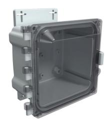
AttaBox Heartland series enclosure, NEMA 1/3R/4/4X/12, 6 x 6 x 4in (HxWxD), wall mount, polycarbonate, Pantone 7541 C light gray, smoked polycarbonate single-door, polycarbonate quick-release latch.
