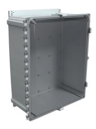
AttaBox Heartland series enclosure, NEMA 1/3R/4/4X/12, 20  $\times$  16  $\times$  8in (HxWxD), wall mount, polycarbonate, Pantone 7541 C light gray, smoked polycarbonate single-door, polycarbonate quick-release latch.
