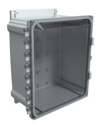
AttaBox Heartland series enclosure, NEMA 1/3R/4/4X/12, 12  $\times$  10  $\times$  6in (HxWxD), wall mount, polycarbonate, Pantone 7541 C light gray, smoked polycarbonate single-door, polycarbonate quick-release latch.
