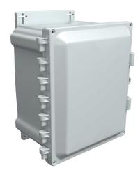
AttaBox Heartland series enclosure, NEMA 1/3R/4/4X/12, 10 x 8 x 6in (HxWxD), wall mount, polycarbonate, Pantone 7541 C light gray, single-door, polycarbonate quick-release latch.
