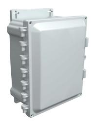
AttaBox Heartland series enclosure, NEMA 1/3R/4/4X/12,  $10 \times 8 \times 4$ in (HxWxD), wall mount, polycarbonate, Pantone 7541 C light gray, single-door, polycarbonate quick-release latch.
