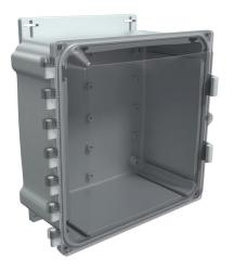
AttaBox Heartland series enclosure, NEMA 1/3R/4/4X/12, 10 x 10 x 6in (HxWxD), wall mount, polycarbonate, Pantone 7541 C light gray, smoked polycarbonate single-door, polycarbonate quick-release latch.
