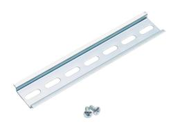
AttaBox DIN rail, slotted, 35mm width, 7mm height, 6.9in length, plated steel. For use with AHx864xxx, AHx884xxx, and AHx108xxxx Heartland series enclosures.
