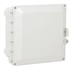
AttaBox Heartland series enclosure, NEMA 1/3R/4/4X/12, 8 x 8 x 4in (HxWxD), wall mount, polycarbonate, Pantone 7541 C light gray, single-door, polycarbonate quick-release latch.
