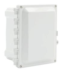
AttaBox Heartland series enclosure, NEMA 1/3R/4/4X/6P/12, 8 x 6 x 4in (HxWxD), wall mount, polycarbonate, Pantone 7541 C light gray, hinged screw cover.
