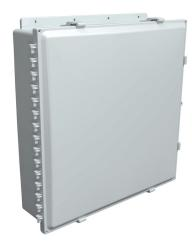
AttaBox Heartland SL series enclosure, NEMA 1/3R/4/4X/12, 24 x 24 x 6in (HxWxD), wall mount, polycarbonate, Pantone 7541 C light gray, single-door, polycarbonate quick-release latch.
